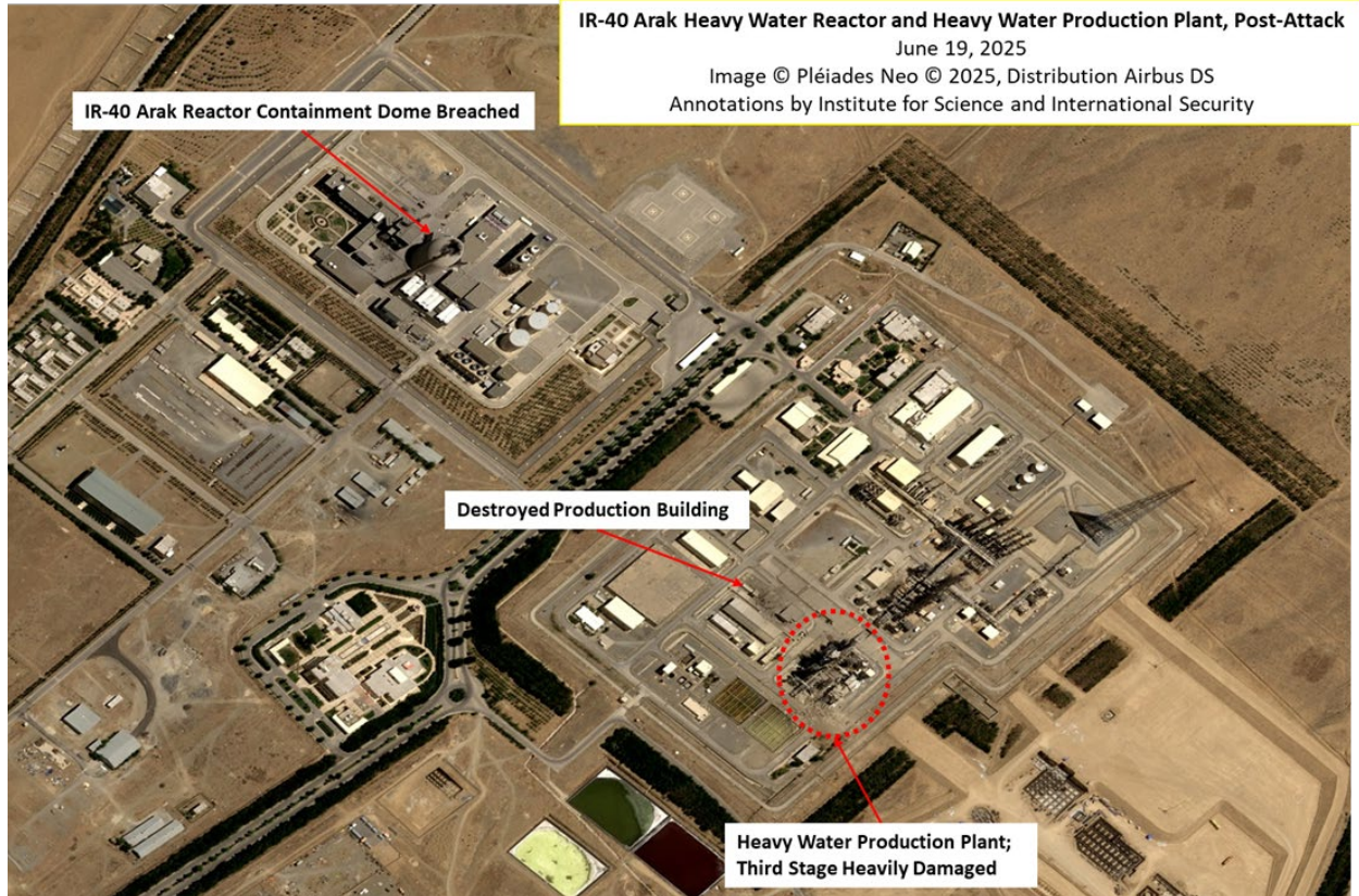
Figure 16. An overview satellite image from June 19, 2025, of the damage done to the IR-40 Arak Heavy Water Reactor Complex and Heavy Water Production Plant.
